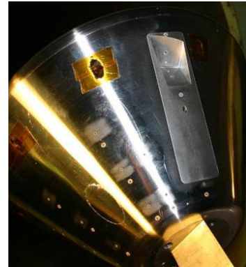
Figure 29. CAD Model of Cavity/RCS Jet Interaction Insert Installed in Spherical Capsule Model
