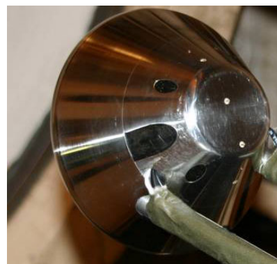
Figure 35. Small-scale Spherical Capsule Model with 5.75" Major Diameter Installed in Facility
