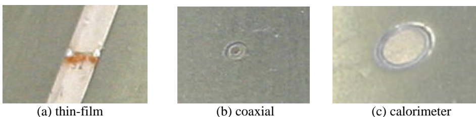
Figure 5. Photos of Types of Heat Transfer Instrumentation employed in LENS Facilities at CUBRC
